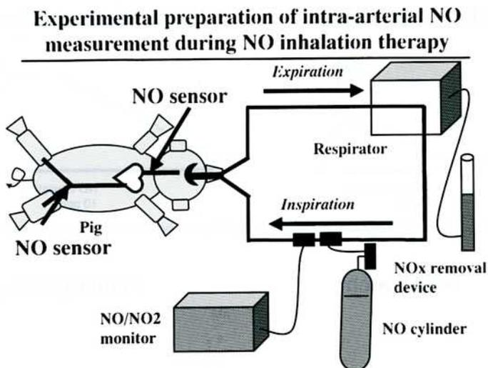
Fig. 2. Locations of two NO sensors (aortic arch and femoral artery)
