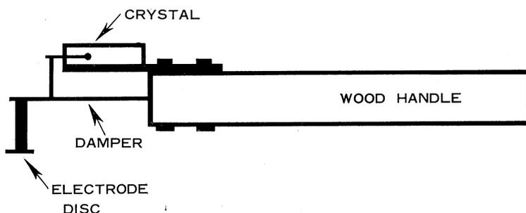
Fig. 1. Transducer-stimulating electrode assembly.
