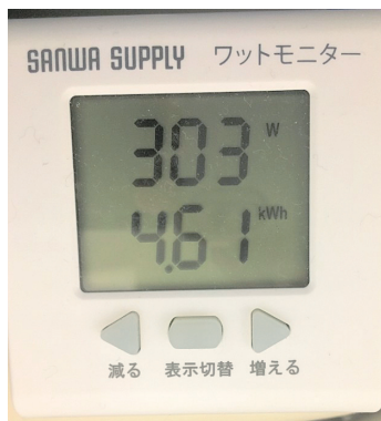
Fig.14 : Power consumption when performing parallel calculations is 303 W. The lower numbers indicate the amount of power.
