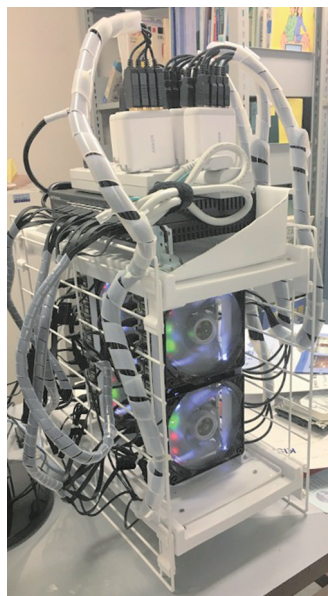
Fig.1 : PIs consisting of 23 Banana Pis and 1 Raspberry Pi on which it is possible to implement the MPI.
