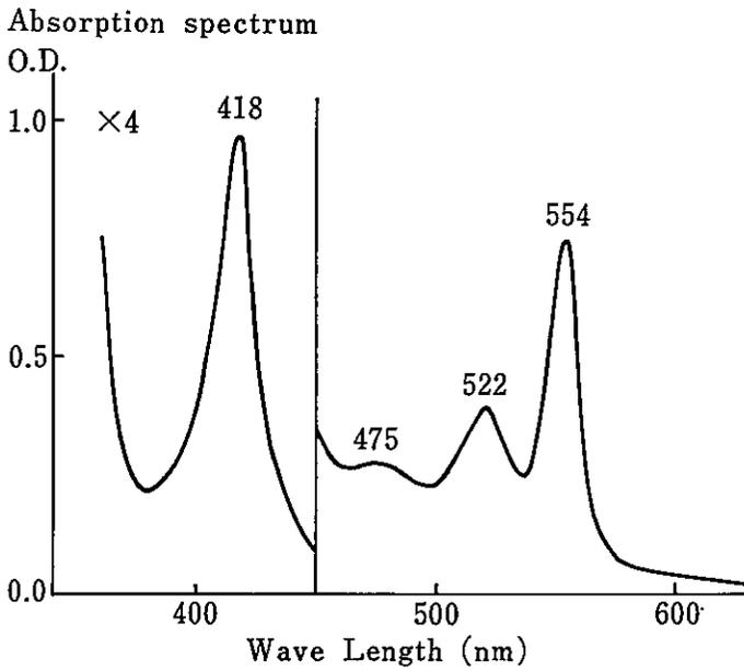
Fig. 3. Absorption curve of the colored solution in the pyridine hemochrome method
