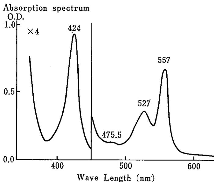
Fig. 1. Absorption curve of the colored solution in the alkali-hemochrome method
