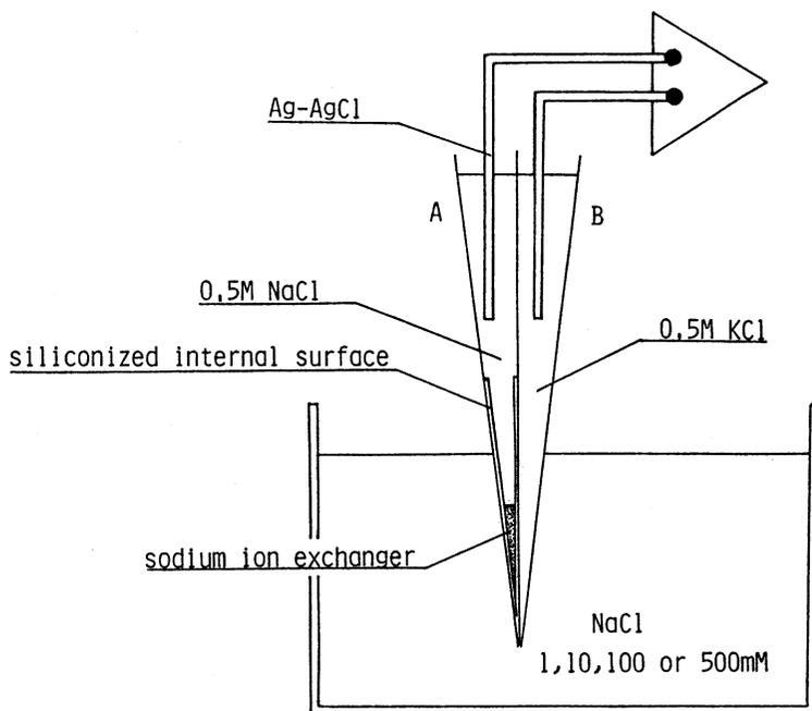
Fig. 1. Schematic diagram of the  $\text{Na}^+$  sensitive double-barrelled glass microelectrode
